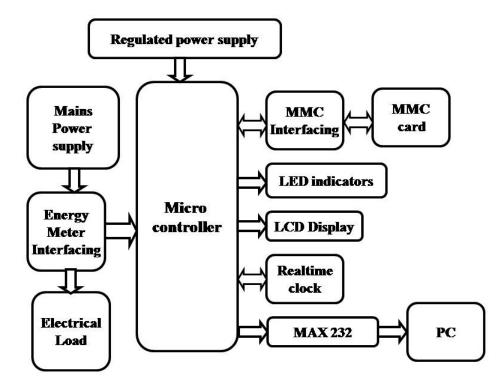
Data logger for energy meter with time and KWH Readings
